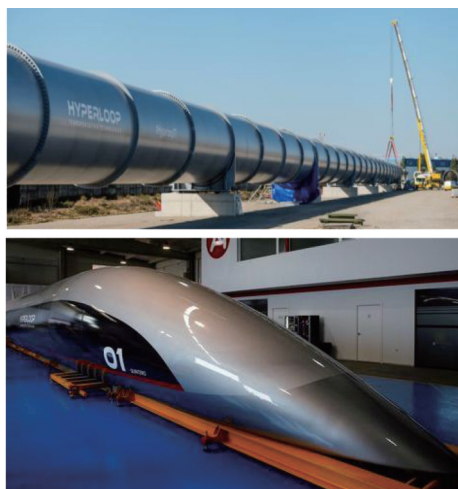
图1 HTT测试轨道和全尺寸列车Quintero One [12]
