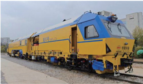
图1 DWL-32 连续式双枕捣稳车 Fig. 1 DWL-32 continuous dual-sleeper tamping and stabilizing vehicle
